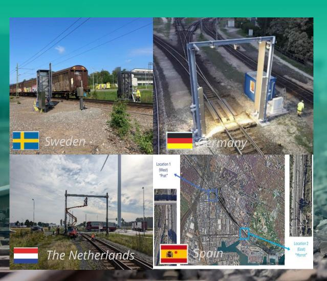
Capturing logistic and maintenance data through a gate equipped with cameras and RFID reader
